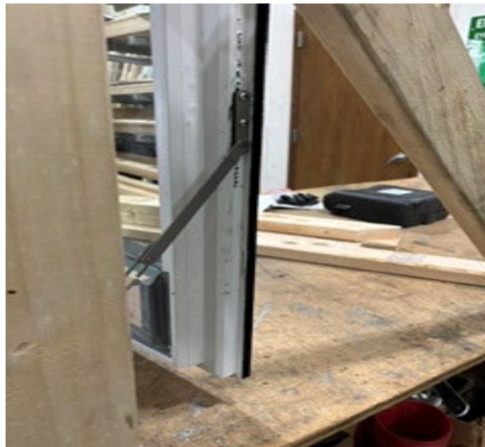
Photo No. 4 WOCD attached to Sash.
